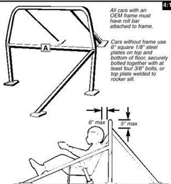
Maximum of 6" from roll bar to driver's helmet. Maximum of 5" from top of roll bar to brace.
